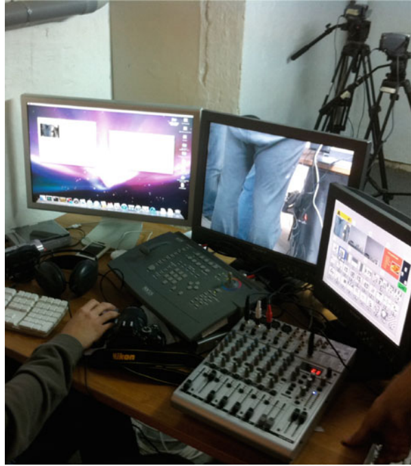
Fig. 2 The iMediaTV control panel featuring the audio mixer, the video mixer, the server and cameras that connects to the video mixer and the direct video server
